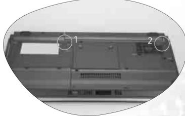
9. Place the battery on its original position and then slide the battery retainer 1 to the right to lock the battery. Connect the AC adapter. When you start Joybook, it will automatically test and configure the new memory.
